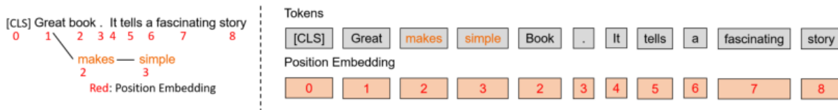
Figure 4: Continuing the example in Figure 2b, we inject the fact triplet ( great , makes , simple ) to the main sentence forming a tree structure (left). On the right, we flatten the tree into a sequence and use the depth of the tokens in the tree as their position embedding index. The highlighted words in orange are the injected fact.
